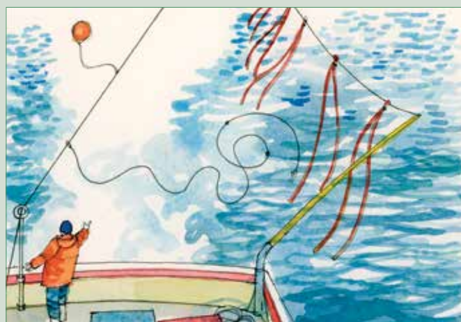
Figure 1. Streamer lines are an example of a cheap seabird bycatch mitigation measure, which can be used in combination with other measures to great effect.
