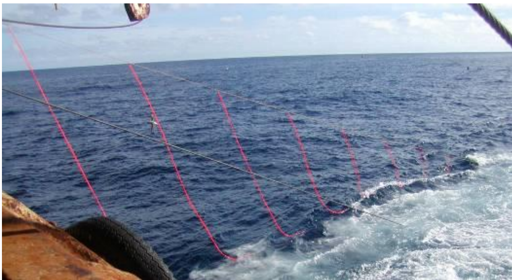
Figure 7. Streamer line with 30 m backbone, Kraton streamers at 3 m intervals, and a mesh-covered 360 mm-diameter trawl float as the terminal object. The starboard trawl warp is also visible (and the port warp crosses the photo in the upper right corner).
