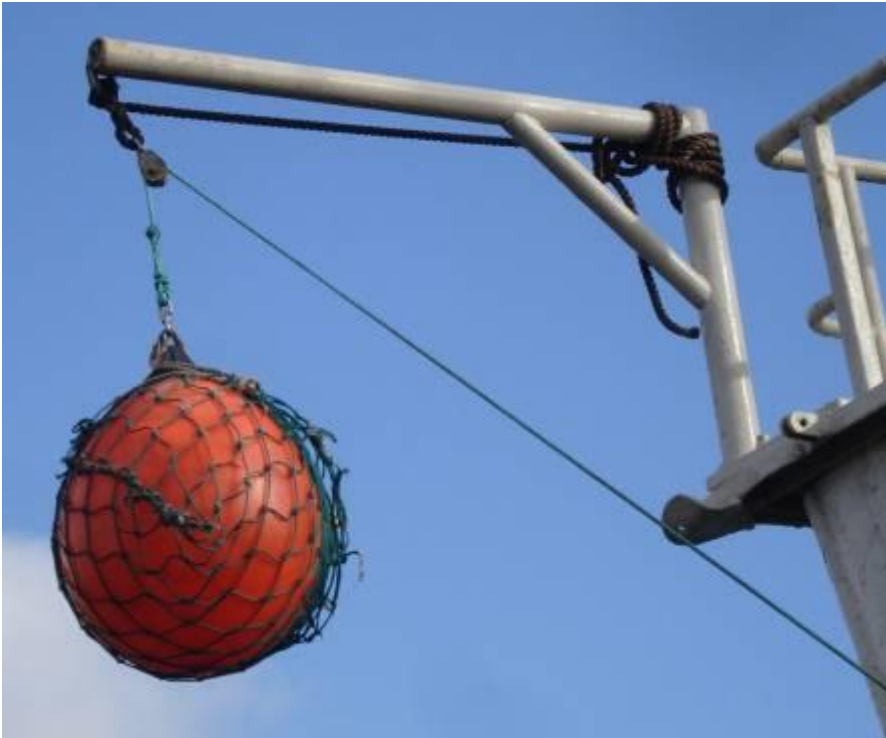
Figure 4. System used to deploy streamer lines on Korean-operated trawl vessels. The buoy is released with a lazy line, drops to the water surface, and pulls the streamer line out as it trails onto the water surface.
