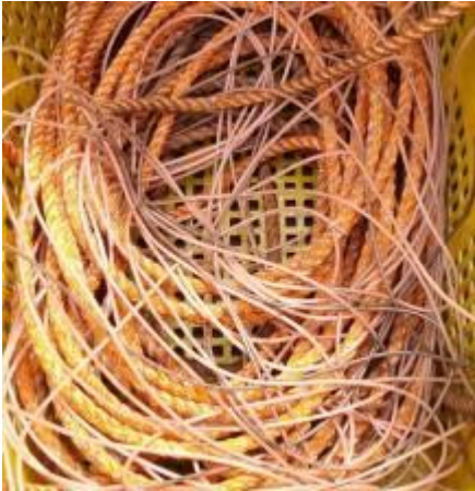
Figure 2. The luminous tubing typically used in streamer lines currently deployed on trawlers \geq 28 m operating in New Zealand waters. Figure 1(a) shows this material when new. Here, the material is shown after 10 days at sea, highlighting the extent of fading that occurs in relatively short timeframes.
