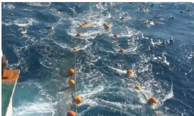
Figure 2: Headline creating pooling area at the stern of the vessel
