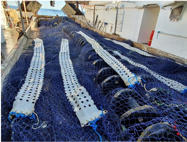
Figure 8: Wide white strips attached to upper panels
