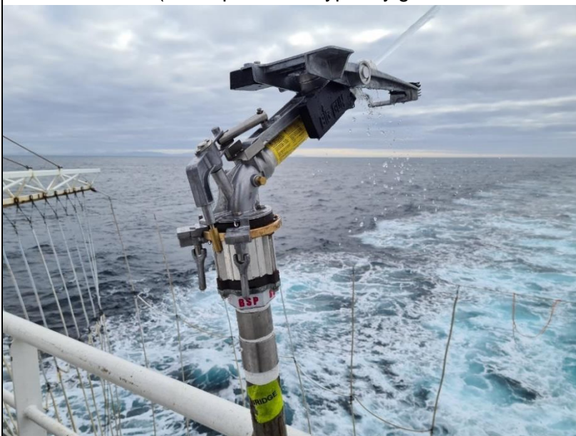
Figure 6: High-pressure water sprayer installed on vessel
