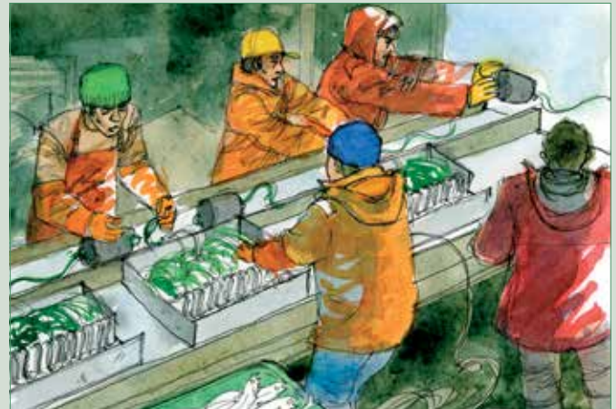
Figure 2. Pushing weights from the setting table and using metal lined boxes helps to reduce tension and improve line sink rate.
