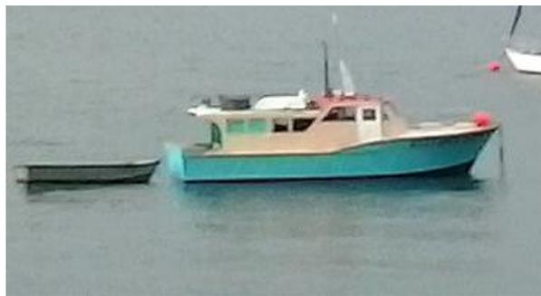
Figure 1. A small bottom longline vessel that is low to the water and has minimal deck structure at the stern for the robust attachment and effective elevation of a tori line. Photo: D. Goad.
