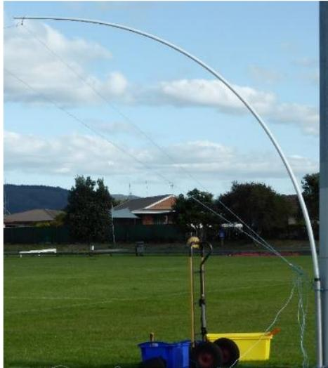
Figure 6. A tori pole under 20 kg of drag - more than was ever required to achieve an aerial extent of 80 m during the on-land trials.
