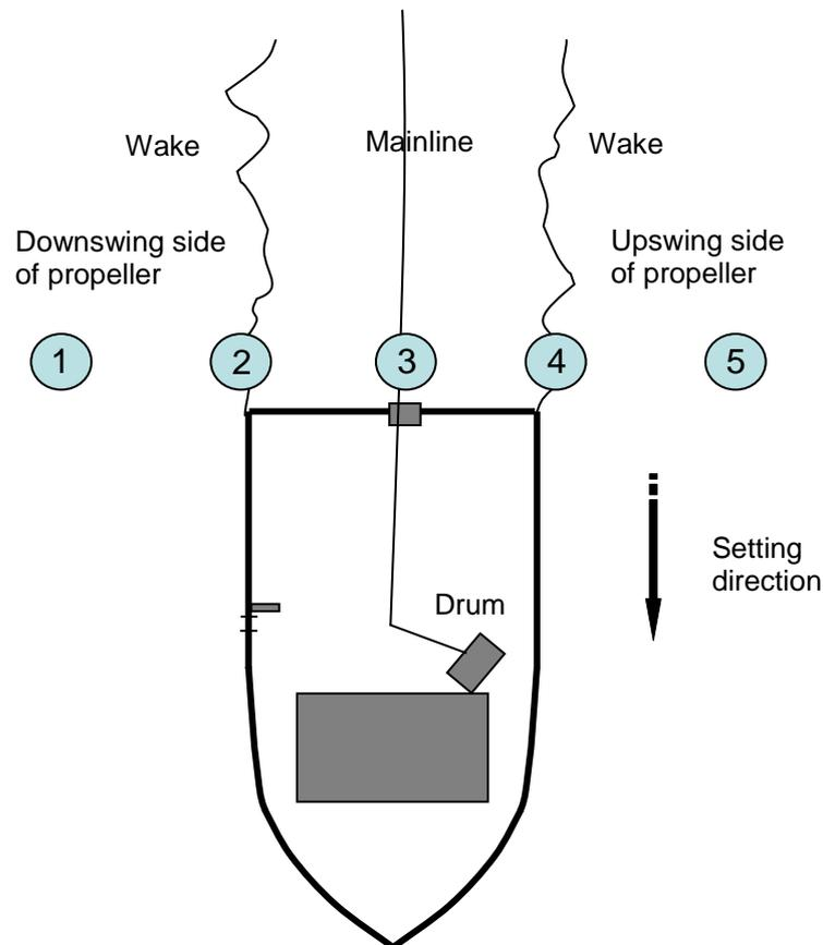
Figure 1. Schematic presentation of the five bait landing positions in proximity to the propeller turbulence assessed in the experiment. In the text the positions are referred to as 1) starboard far; 2) starboard wake; 3) centre; 4) port wake; and 5) port far.
