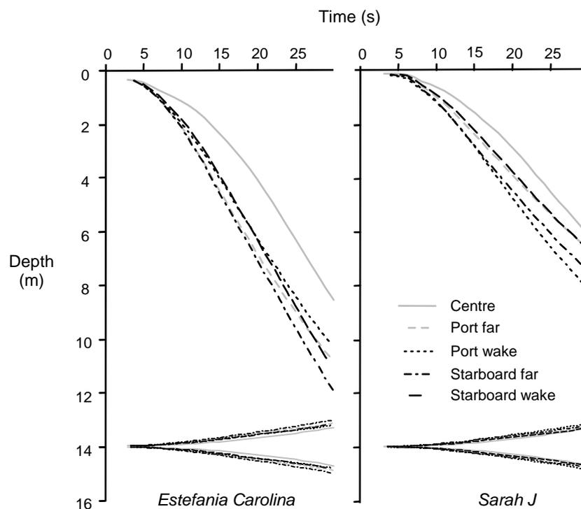
Figure 2. Comparison of sink profiles of baited hooks set from the F/Vs *Estefania Carolina* and *Sarah-J* in the five bait landing positions related to propeller turbulence. The comparison is based on the swivel first branch line deployment method, which was the method common to both vessels.
