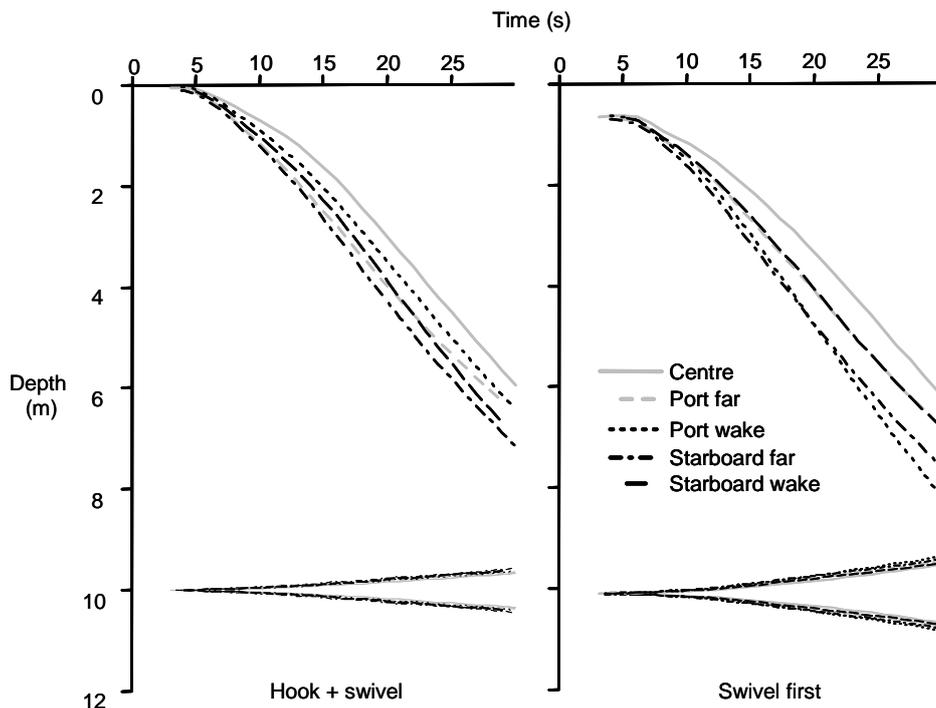
Figure 3. Comparison of bait landing positions within branch line throwing method in relation to turbulence from the propeller of the *Sarah-J*. The profiles for the swivel first method are identical to those for the *Sarah-J* in Figure 2, but appear slightly different because of the different scales on the depth axis of both graphs.
