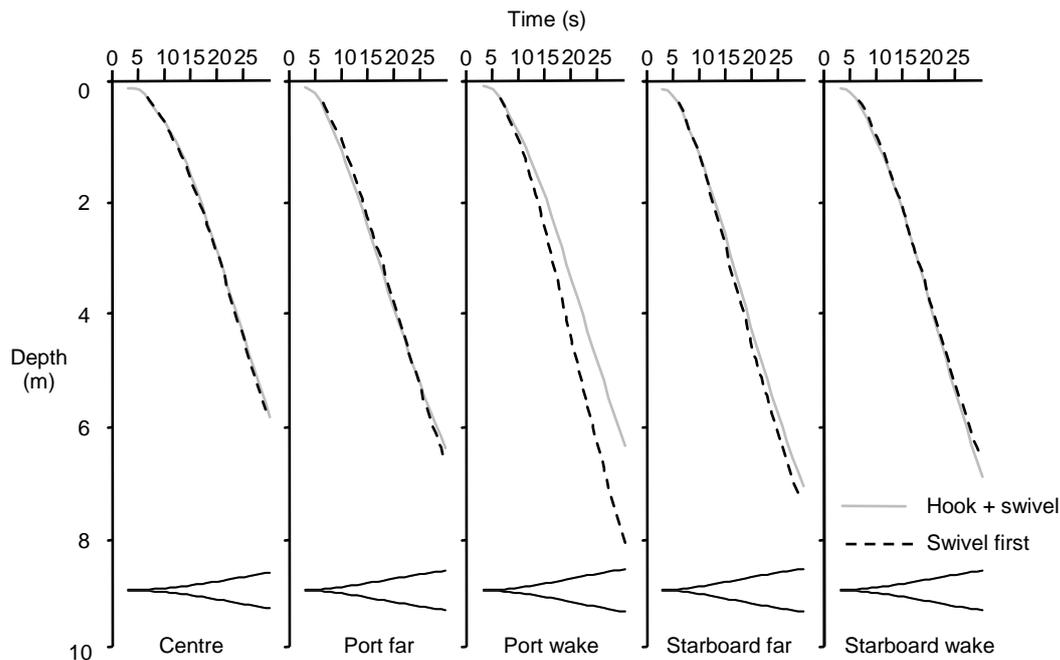
Figure 4. Comparison of bait throwing method within the five bait landing positions in relation to thrust from the propeller of the F/V Sarah-J.
