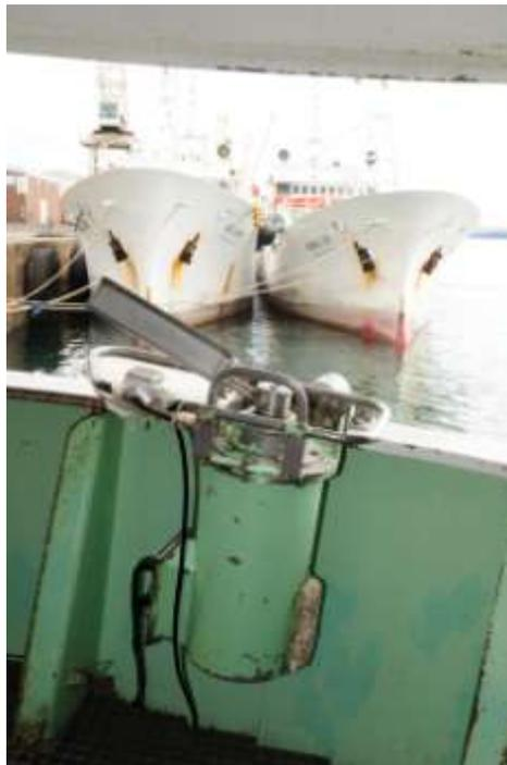
*Figure 1. Bait casting machine fitted to a high seas-type tuna vessel in Cape Town, South Africa. Baited hooks are placed in the rectangular container (projecting at left) which rotates at high speed in a clockwise direction, casting baits in a direction to the right of the picture.*
