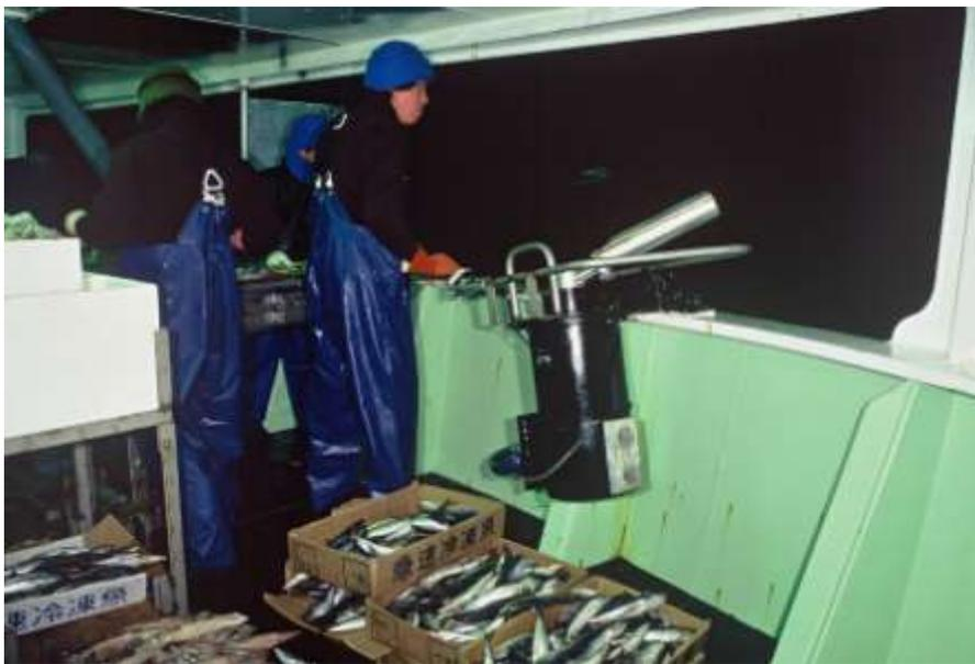
*Figure 2. Japanese-made “Tuna Mate” bait casting machine in operation on a Japanese tuna vessel fishing out of Hobart (under the CCSBT agreement) in the mid 1990’s. Still photography does not impart an accurate impression of the velocity of the cast which, in this case, straightened the 40 m branch line. Baited hooks landed in clear (un-aerated) water 15-20 m outboard of the streaming position of the bird scaring streamer line.*
