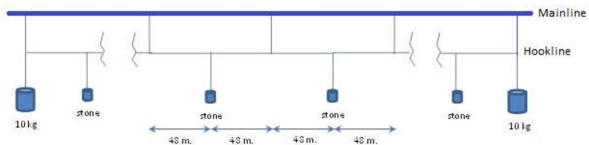
Figure 1: Namibian demersal longline gear configuration
