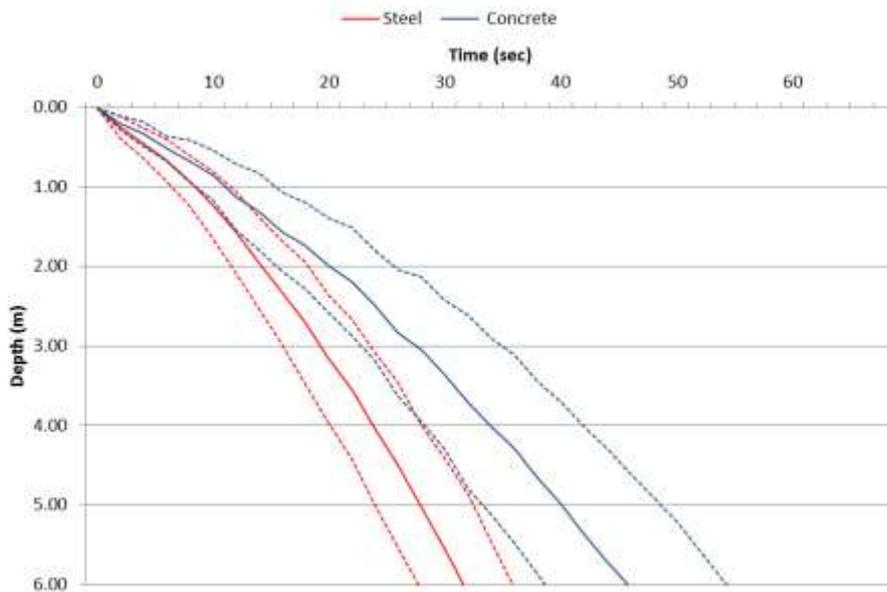
Figure 3: Mean sink rate profiles plus standard deviation of the slowest sinking longline sections for each treatment (concrete and steel weights).
