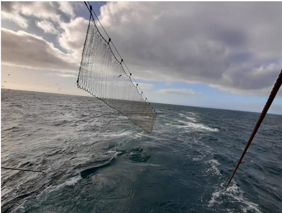
Figure 3. Netsonde curtain for the middle and lower section of the netsonde cable (upper plate showing deployment and final weighted blocks for netsonde curtain) (© ATF-Chile).
