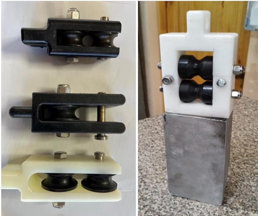
Figure 4. Evolution in block designs for netsonde curtain deployment. For use along the curtain, it is recommended to have double blocks with Teflon wheels, where one of them can have a lock to facilitate removal and replacement (left-bottom). If it is necessary to support the proper deployment of the curtain, the use of systems with added weights in the lower section of the curtain is recommended, such as attached chains, or alternatively, installing blocks with added weight on the block rail that deploys the curtain above the water level, thus facilitating its deployment along the middle and lower 2/3 of the netsonde cable (see right image, 10 kg for reference).
