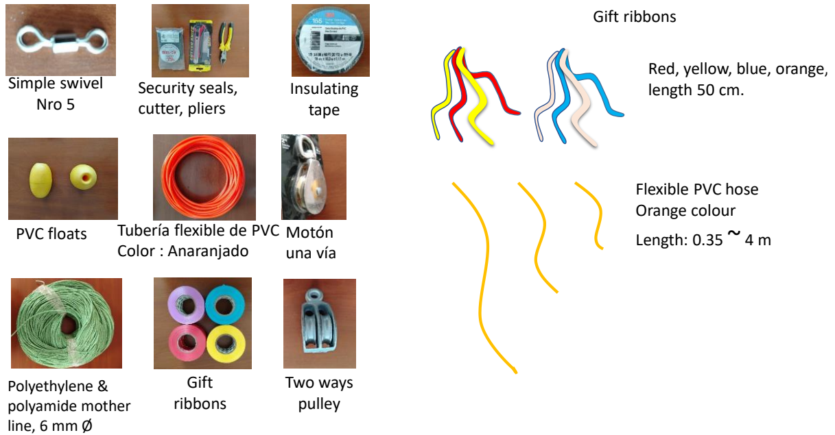
Fig. 5. Local materials employed to the construction of the Peruvian version of the Tori Line.
