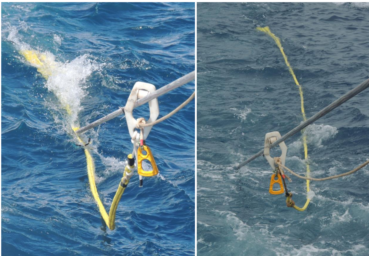
Figure 1: Scheme of the assembly of the bird scaring line specially designed for the net monitoring cable composed of three elements: a Nylon rope, a Teflon block, and a second Polysteel rope with positive buoyancy. Figures 2 and 3: two images showing the operation of the bird scaring line, the first one near the net monitoring cable and the other further away.
