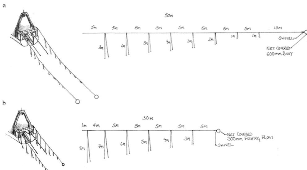
Figure 1: Schematic and dimensions of BSL designs (a) BSL-2004 and (b) BSL-2008
