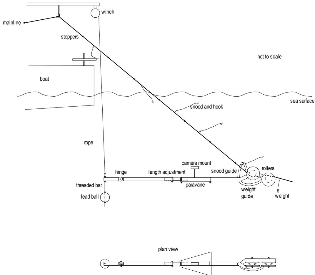
**Figure 9.** Prototype of underwater setting device developed by Dave Kellian.
