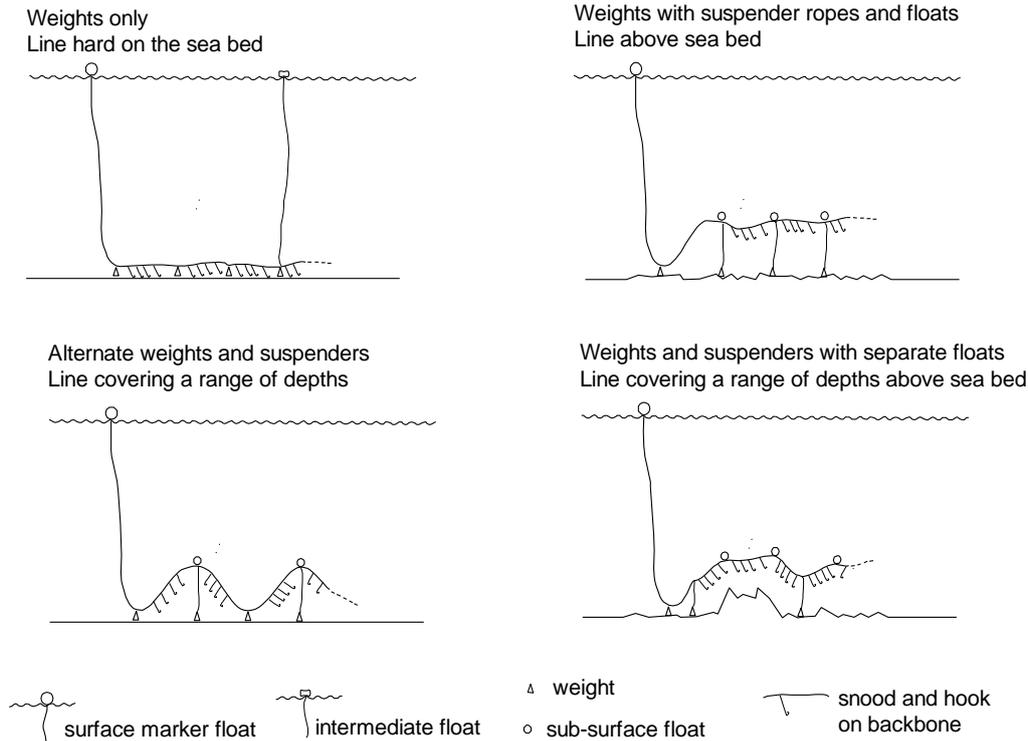
**Figure 1.** Example line configurations.
