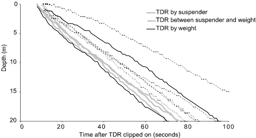
**Figure 4.** Time-depth profiles for TDRs on a typical snapper set. The two slowest sinking TDRs were within 50 m of a surface float.
