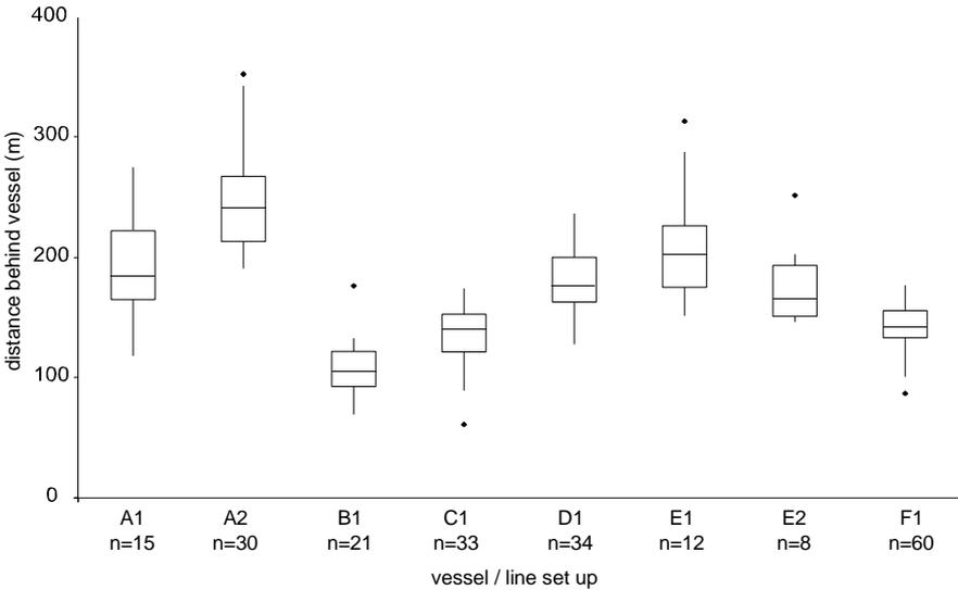
**Figure 5.** Distance behind the vessel that TDRs reached 15m depth, for 8 different line set ups tested during normal fishing operations. B1 had the most weighting (5 kg per 100 m), A2 the least (1 kg per 100 m).
