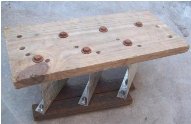
Figure 3: The towed device with 400g weights attached to the lower surface of the keels
