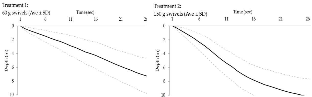
Figure 9: Sink rate profiles (mean  $\pm$  SD) for Treatment 1 (60g) and Treatment 2 (150g) safe leads
