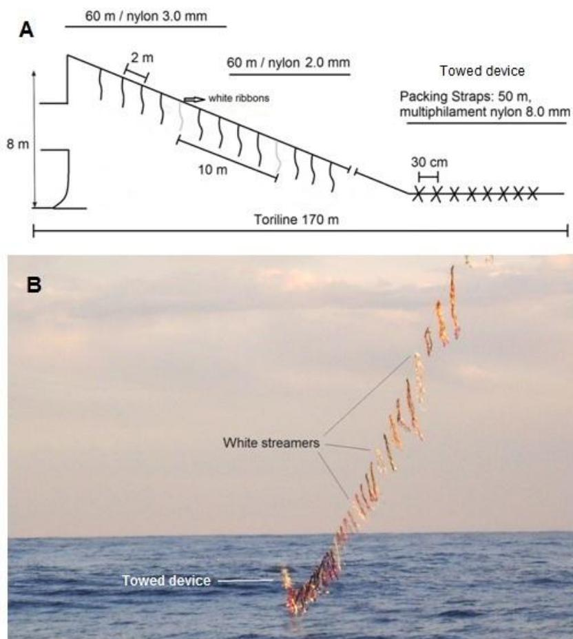
Figure 1: (A) Schematic picture of the Brazilian tori line. (B) Tori line *in situ* aboard the FV Akira V.
